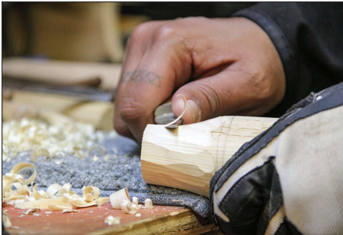
It takes Myles an hour to shape a handle, which is custom fit to each paddle.
